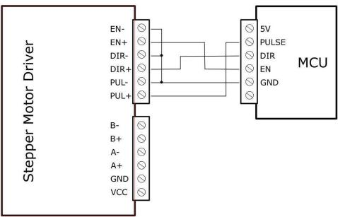
Note: When "EN" is in the valid state, the motor is in a free states (Off-line mode). In this mode, you can adjust the motor shaft position manually.
