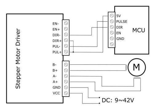
Note: Please cut off the power when you connect the system, and ensure the power polar is correct. Or it will damage the controller.
